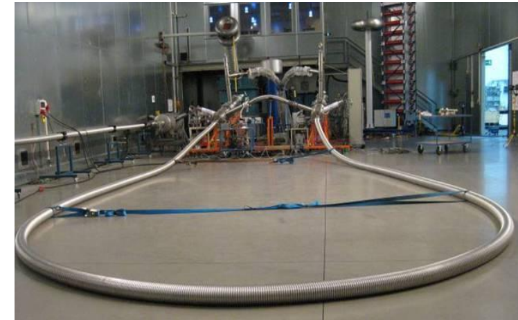
HTS cable 24kV-3200 A (Nexans). 2012 Premi ENDESA – Novare a ICMAB
